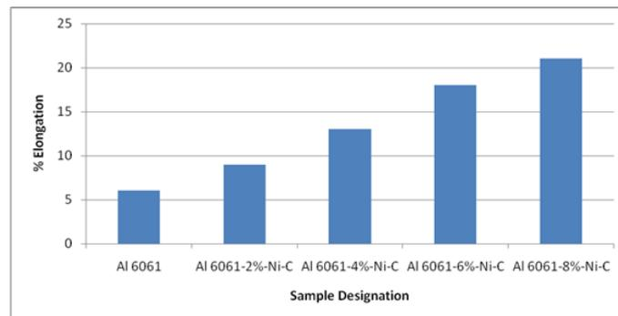
**Figure 3** Variation of ductility (%age elongation) of Al 6061 matrix alloy and the developed nickel coated cenosphere composites
