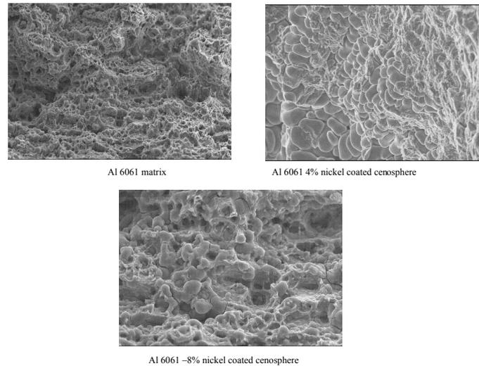
**Figure 4** Fractographs of Al 6061 alloy and the developed nickel coated cenosphere composites
