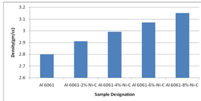
**Figure 1** Variation of density of Al 6061 alloy and Al6061-nickel coated composites
