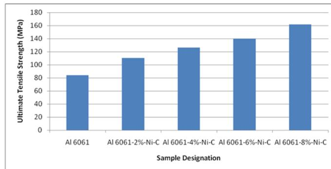
**Figure 2** Variation of Ultimate Tensile strength of Al 6061 matrix -nickel coated cenosphere and the developed composites
