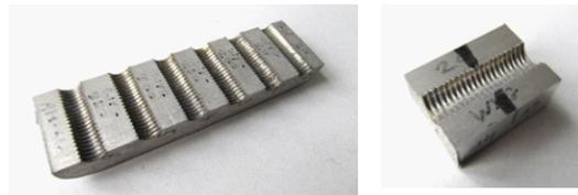
**Figure 3** Samples of threads made in magnesium alloy – view of cross – section after wire cutting
