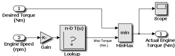
Figure 6: Engine torque control
