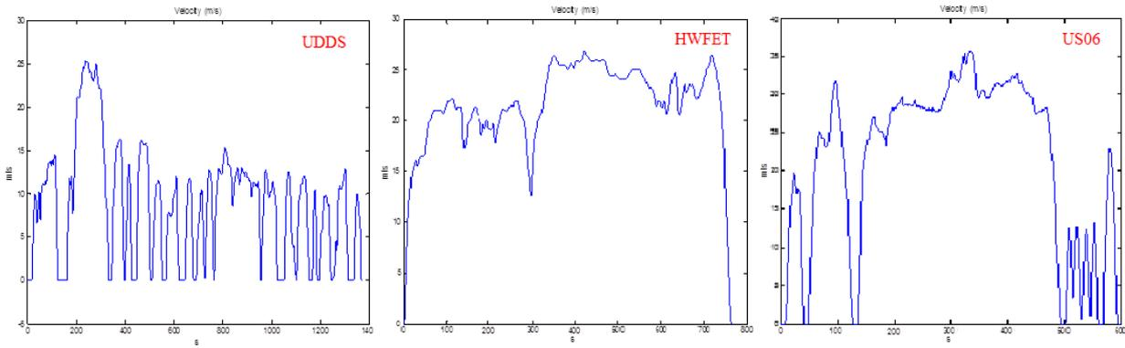
Figure 16: Actual velocities and desired velocity versus time for UDDS, HWFET, and US06
