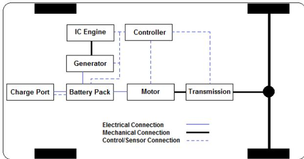
Figure 1: Plug-in series powertrain
