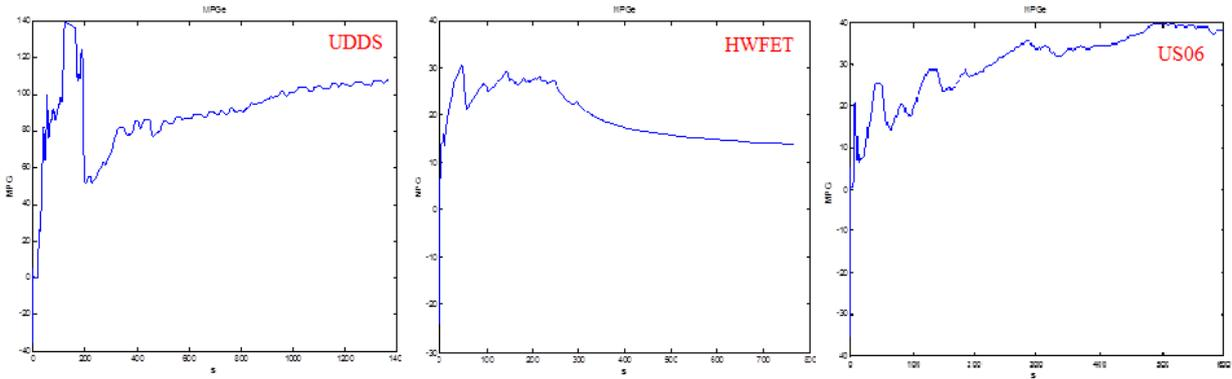
Figure 17: MPGe versus time UDDS, HWFET, and US06
