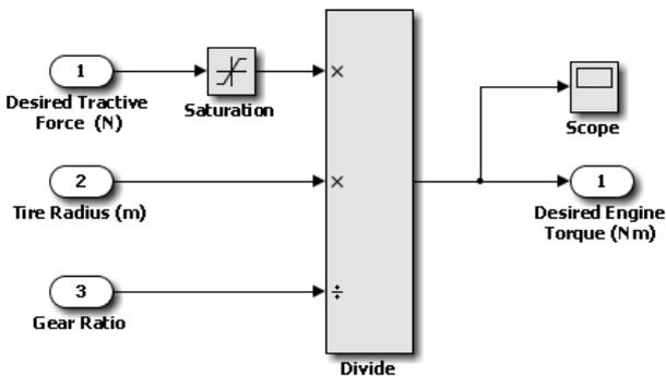
Figure 5: Engine torque model
