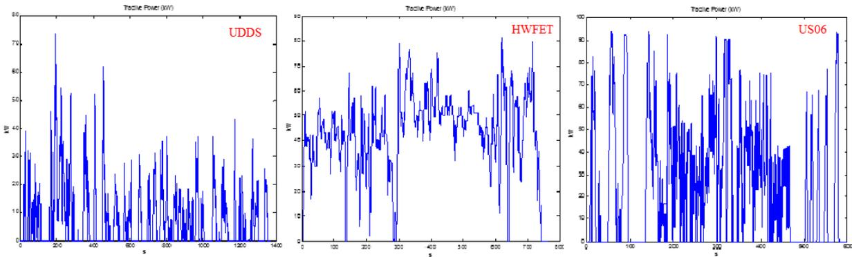
Figure 18: Tractive power (in kWh) versus time for UDDS, HWFET, and US06
