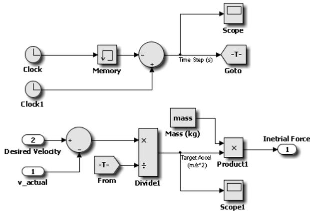
Figure 3: Inertia force (N)
