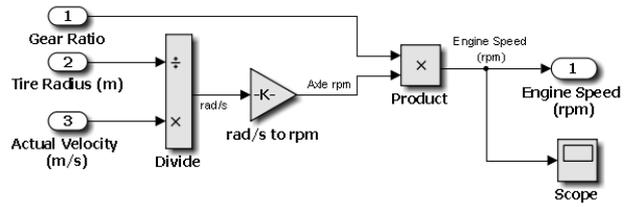
Figure 7: Engine speed calculation
