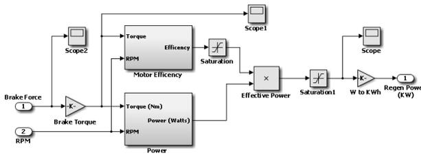
Figure 13: Braking or deceleration model
