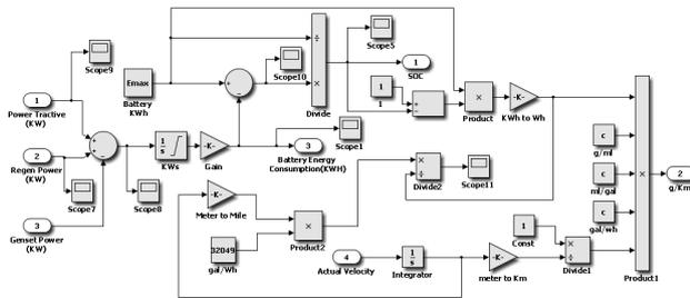
Figure 14: Battery model
