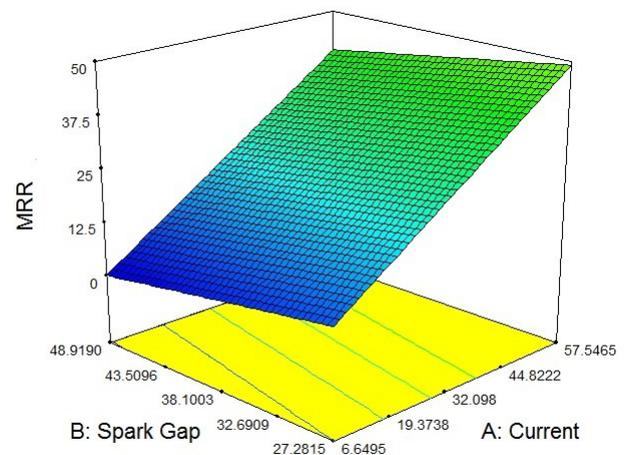
**Figure 3:** Effect of spark gap versus current on MRR
