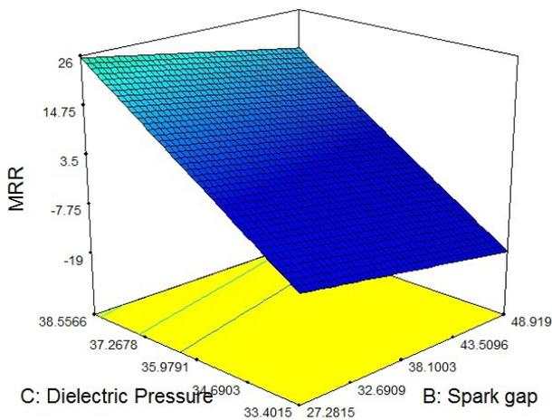
**Figure 4:** Effect of spark gap versus dielectric pressure on MRR
