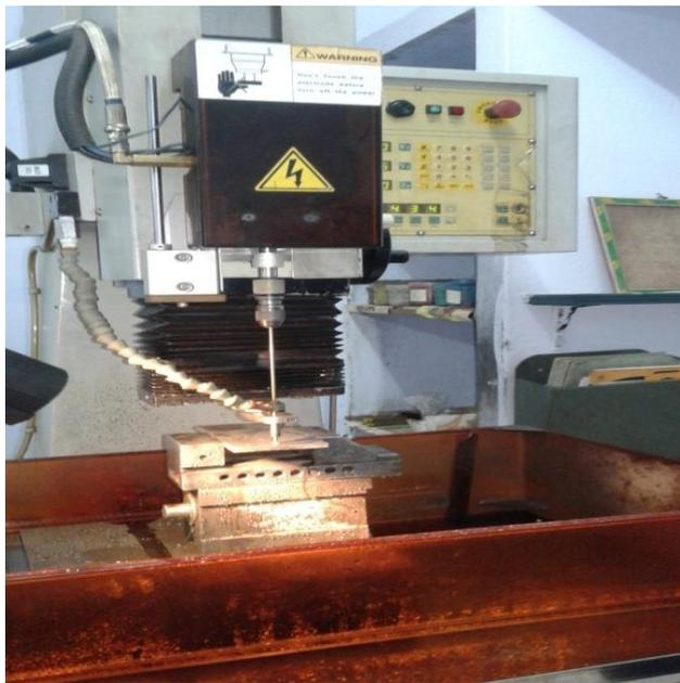
**Figure 1:** Electric discharge machine
