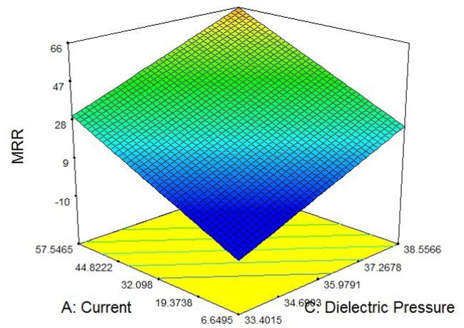
**Figure 2:** Effect of current versus dielectric pressure on MRR
