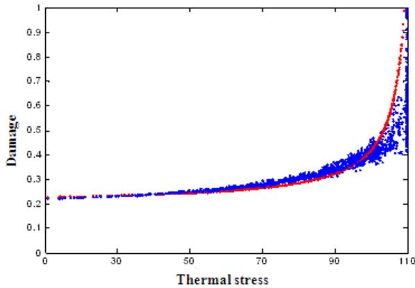
Figure 7: The influence of thermal stress on the interface damage ( $\sigma = 115 \text{ N/m}^2$ )
