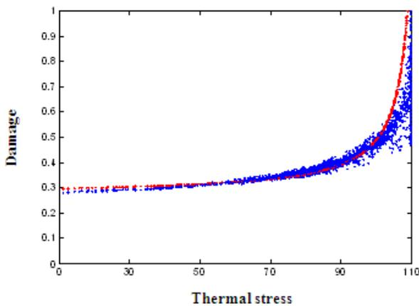
Figure 3: The influence of the thermal stress on the interface damage ( $\sigma = 105 \text{ N/m}^2$ )
