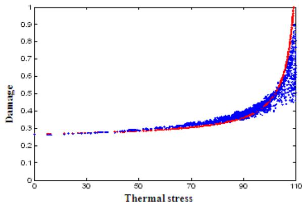
Figure 8: The influence of thermal stress on the interface damage ( $\sigma = 125 \text{ N/m}^2$ )
