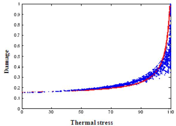
Figure 6: The influence of thermal stress on the interface damage ( $\sigma = 105 \text{ N/m}^2$ )
