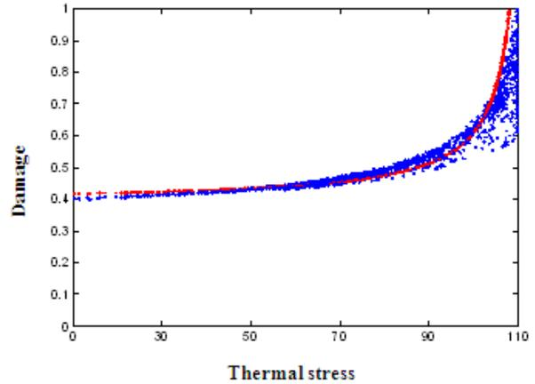
Figure 4: The influence of thermal stress on the interface damage ( $\sigma = 115 \text{ N/m}^2$ )
