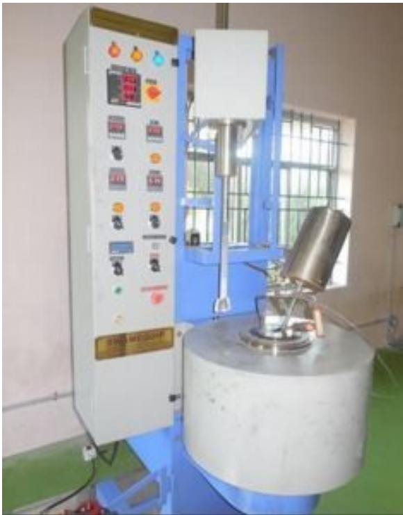
Figure 1: Experimental setup of stir casting
