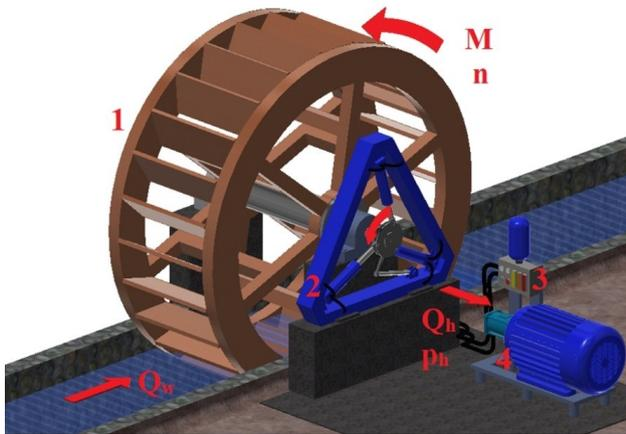
**Figure 1:** Visualization of hydrostatic transmission in a small hydropower plant with input parameters: 1 – water wheel, 2 – radial piston pump, 3 – hydraulic equipment, 4 – hydraulic motor connected to the asynchronous generator.
