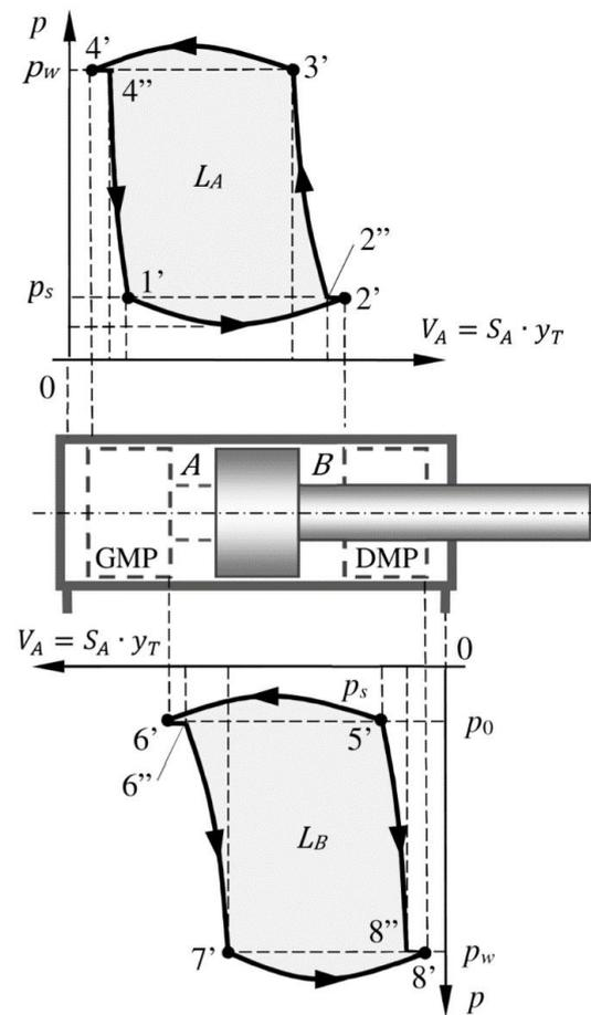
Figure 4: Indicator diagrams of real suction-pressure unit.
