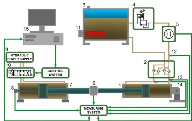
**Figure 6:** Flowchart of the test stand: 1 – suction-pressure unit, 2 – valve timing, 3 – hydraulic oil tank, 4 – pressure relief valve, 5 – flowmeter, 6 – force sensor, 7 – drive actuator, 8 – position sensor, 9 – hydraulic power supply, 10 – servo valve, 11 – heater, 12–14 – pressure sensors, 15 – computer.
