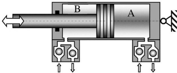
Figure 2: Schematic view of a suction-pressure unit [13].
