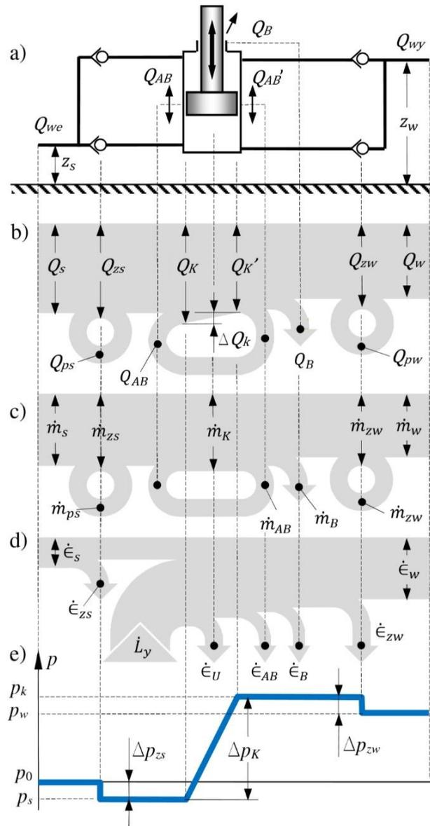
**Figure 3:** Suction-pressure unit: a) functional diagram, b) band chart of volume flux, c) band chart of mass flux, d) band chart of energy, e) pressure change.
