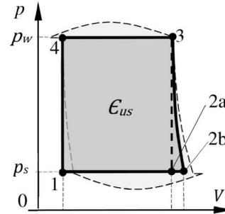
Figure 5: Indicator diagram of useful energy.
