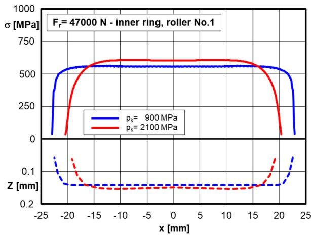
Figure 5: Distributions of von Mises stresses  $\sigma$  and the depth of their occurrence  $Z$  along the line of contact of roller No. 1 with inner ring raceway.
