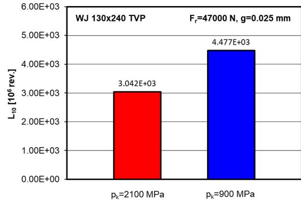
**Figure 9:** The predicted fatigue life of the axle box bearing with modified logarithmic correction of roller generators with parameters determined in accordance with  $p_K = 2100$  MP and  $p_K = 900$  MPa.
