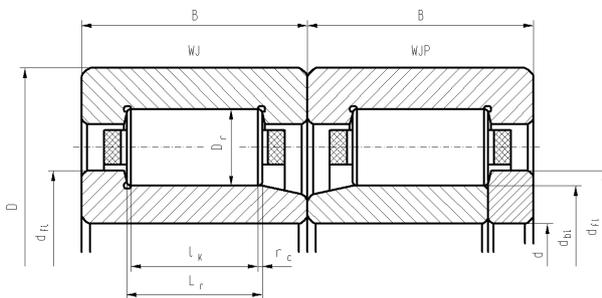
**Figure 1:** Axle box bearings of a two-axle Intercity passenger carriage bogie.
