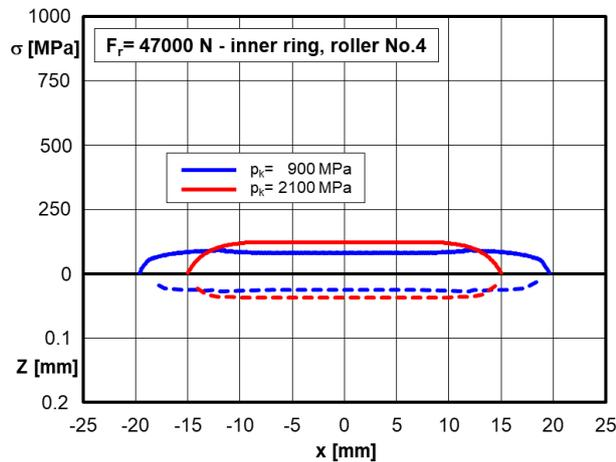
**Figure 8:** Distributions of von Mises stresses  $\sigma$  and the depth of their occurrence  $Z$  along the line of contact of roller No. 4 with inner ring raceway.
