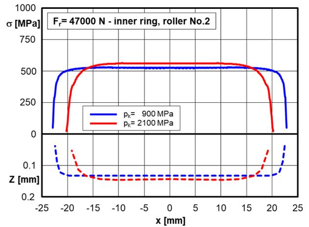
Figure 6: Distributions of von Mises stresses  $\sigma$  and the depth of their occurrence  $Z$  along the line of contact of roller No. 2 with inner ring raceway.
