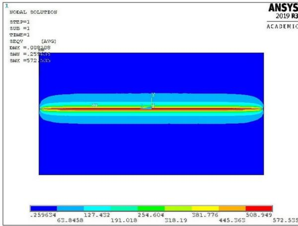
Figure 4: Distributions of von Mises stresses under the most loaded roller-inner ring raceway contact surface,  $p_K = 900$  MPa.
