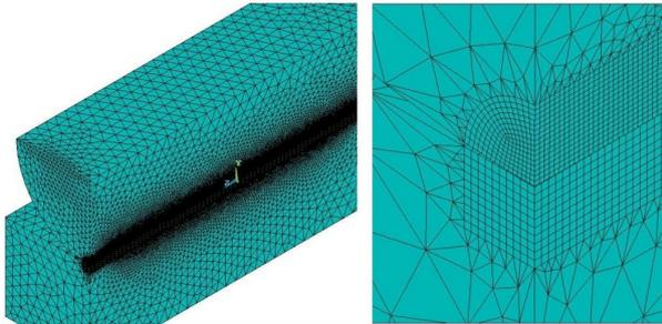
Figure 2: FEM solid model (3D) of the roller-raceway contact.
