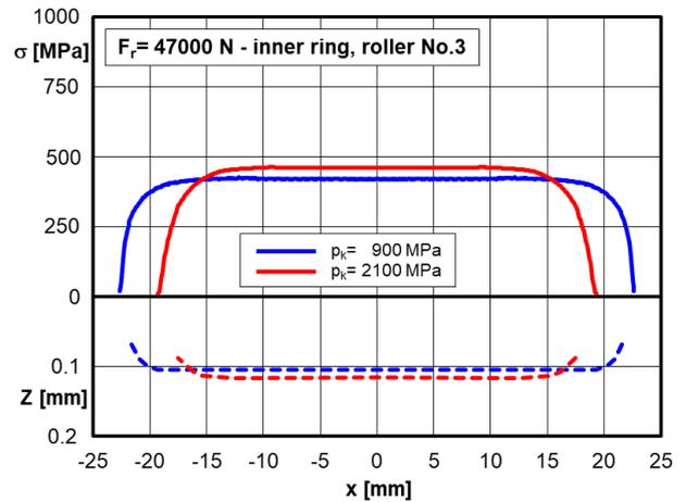
Figure 7: Distributions of von Mises stresses  $\sigma$  and the depth of their occurrence  $Z$  along the line of contact of roller No. 3 with inner ring raceway.
