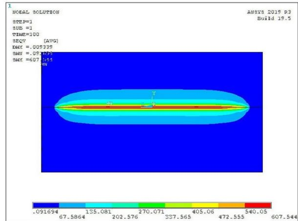
**Figure 3:** Distributions of von Mises stresses under the most loaded roller-inner ring raceway contact surface,  $p_K = 2100 \text{ MPa}$ .
