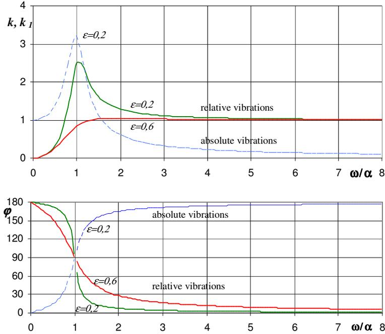
Fig. 1.7. Frequency, amplitude and phase characteristics of the seismic sensor
