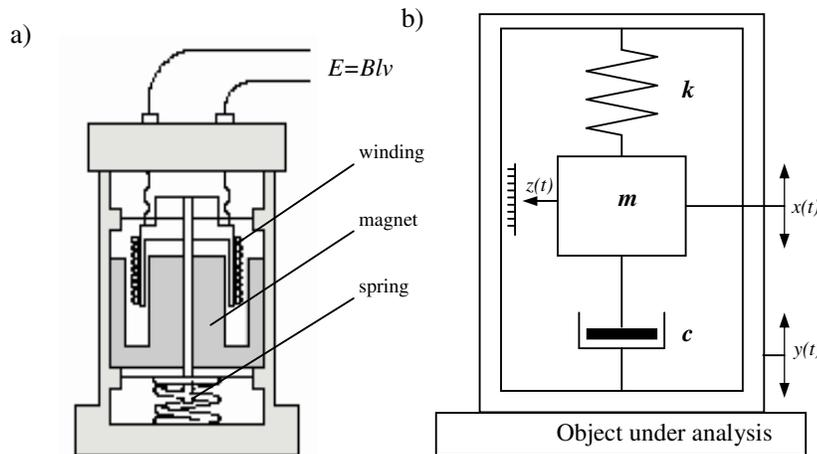
Fig. 1.6. Design and model of the mechanical system of the seismic electro-dynamic sensor
