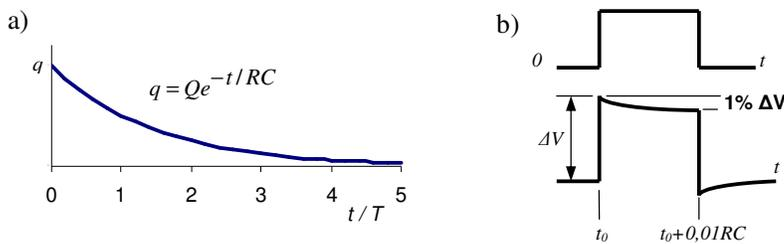
Fig. 1.16. a) discharge curve, b) response to the rectangular excitation
