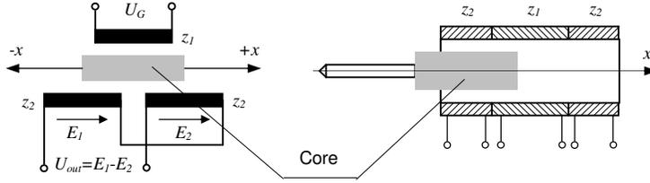
Fig. 1.1. Inductive transformer sensor
