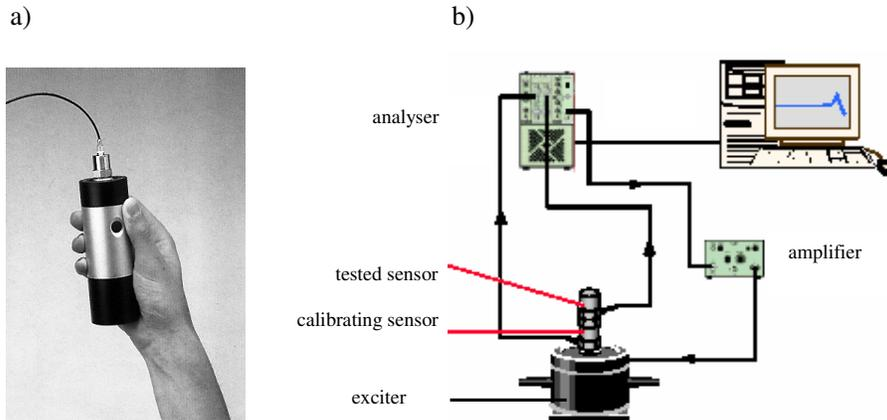
Fig. 1.23. Test of the sensor sensitivity: a) with a transportable calibrator, b) by determining the frequency characteristics with a calibrating exciter (Brüel&Kjær)
