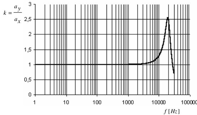
Fig. 1.15. Characteristic curve of the piezoelectric sensor
