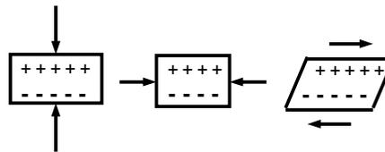
Fig. 1.13. Piezoelectric effects: longitudinal, transversal and shearing
