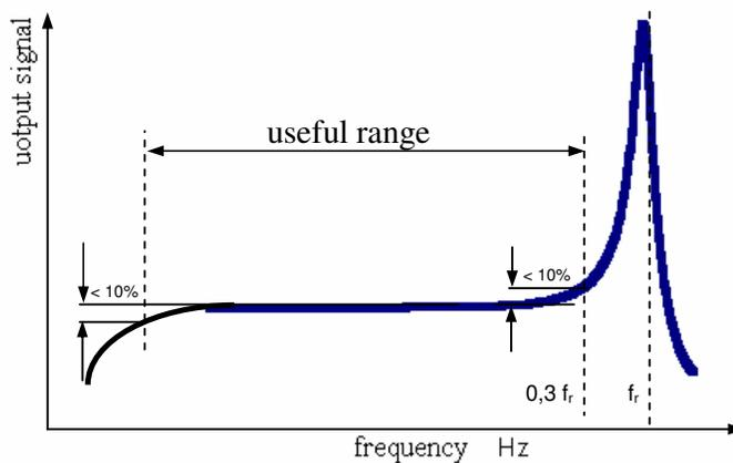
Fig. 1.17. Piezoelectric sensor characteristic
