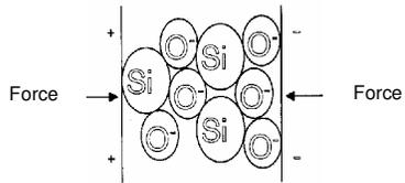
Fig. 1.12. Piezoelectric effect in the quartz crystal grid
