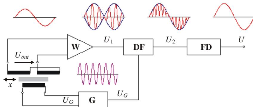
Fig. 1.4. Block scheme of the sensor with phase-sensitive rectification
