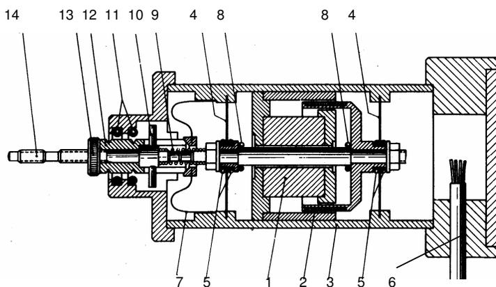
Fig. 1.10. Electro-dynamic sensor, type PR9267 (Philips):
