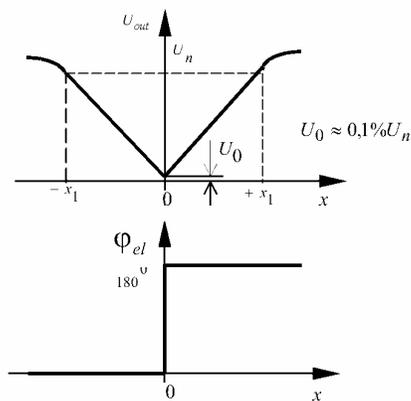
Fig. 1.2. Dependence of the amplitude and phase of the differential transformer sensor on the core displacement
