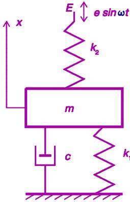
Fig. 4.2. Model of the experimental – equivalent system
