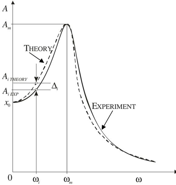
Fig. 4.4. Theoretical and experimental resonance graphs
