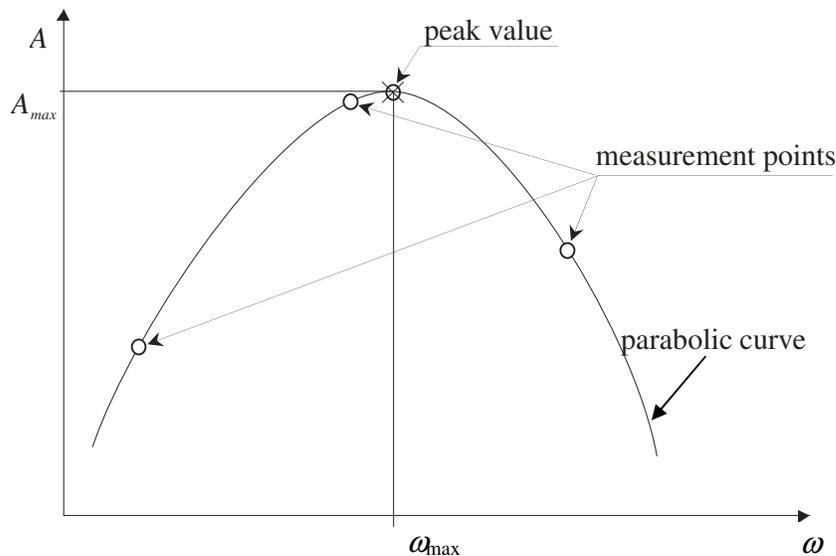
Fig. 4.5. Improved method for finding the peak value of the resonance graph
