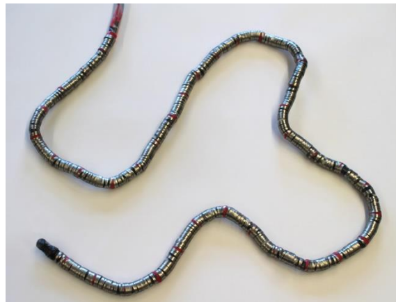
Figure 2 Snake robot based on McKibben PAMs
