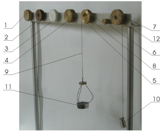
Figure 2: Station for testing string friction and resistance moments
