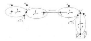
$\textbf{Figure 5} \ \text{Schematic diagram of the RRPR robot with primary particles and the body attached coordinate frames }$
