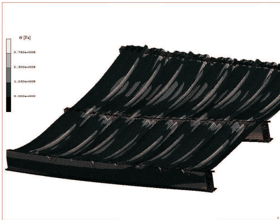
Figure 12 Reduced stress (Mises)
