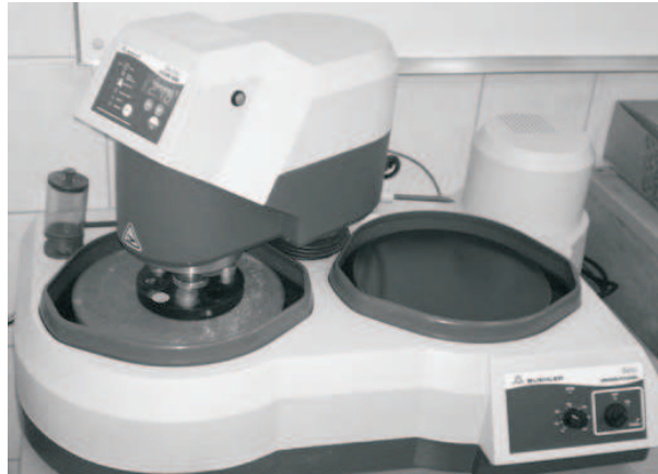
Figure 3 The overall view of the Beta 2 dual platen grinder-polisher machine equipped with Vector power head and specimens holder
