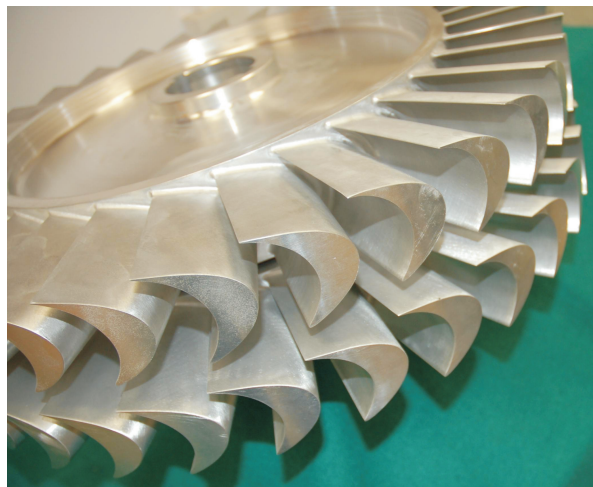
Figure 4 Rotors are manufactured as bladed discs (blisks) out of one piece
