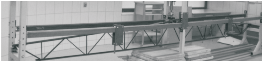
Figure 2 Experimental set-up of truss with elastic braces
