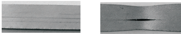
Figure 1 Metallographic specimen of a sheet with visible inclusions
