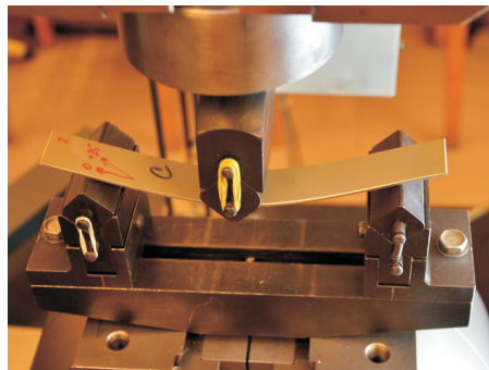
Figure 7 FML specimen during three point bending test
