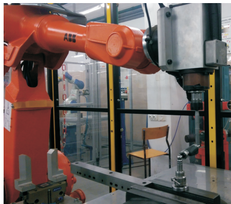
Figure 3 Robot IRB 2400 with telescoping ball bar
