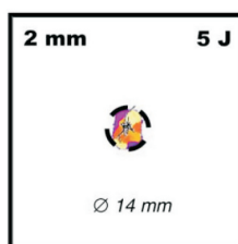
Figure 3 Size of damaged region for 16ply plate impacted with 5J energy [4]
