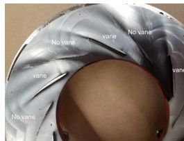
Figure 12 Illustration of the ‘phantom’ diffuser vane effect showing clear flow guidance
